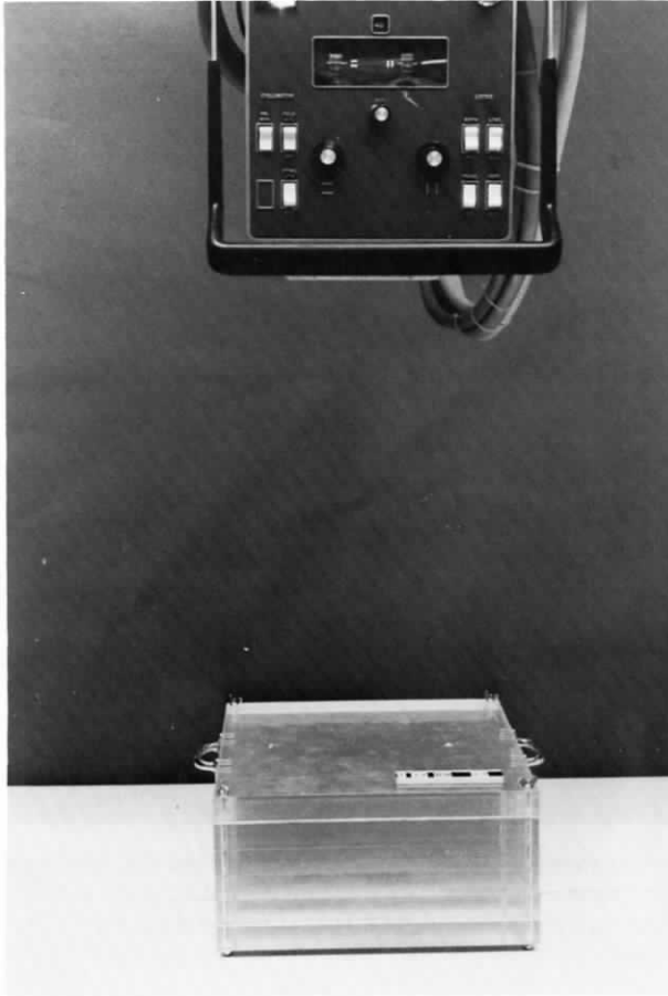
Figure 6.6. Basic homogeneous phantom test setup. The x-ray field should be centered and collimated to the edges of the phantom. A marker indicating the date and room number should be included.
